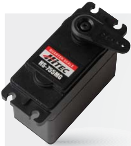
HS-755MG METAL GEAR QUARTER SCALE 4.8 V Torque : 12.0 kg.cm 4.8 V Speed : 0.28 sec/60° 6.0 V Torque : 14.4 kg.cm 6.0 V Speed : 0.23 sec/60° Dimensions : 59 x 29 x 50 mm Weight : 117 g Stock# 32755
