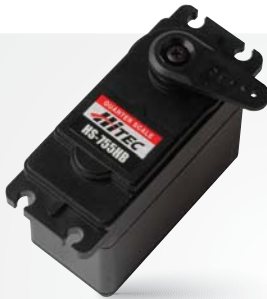
HS-755HB KARBONITE QUARTER SCALE 4.8 V Torque : 11 kg.cm 4.8 V Speed : 0.28 sec/60° 6.0 V Torque : 13.2 kg.cm 6.0 V Speed : 0.23 sec/60° Dimensions : 59 x 29 x 50 mm Weight : 110 g Stock# 33755
