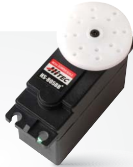
HS-805BB MEGA QUARTER SCALE 4.8 V Torque : 19.8 kg.cm 4.8 V Speed : 0.19 sec/60° 6.0 V Torque : 24.7 kg.cm 6.0 V Speed : 0.14 sec/60° Dimensions : 66 x 30 x 57.6 mm Weight : 152 g Stock# 31805S
