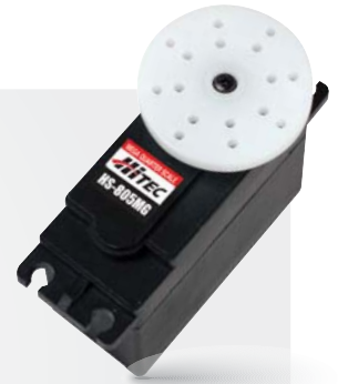
HS-805MG MEGA METAL QUARTER SCALE 4.8 V Torque : 19.8 kg.cm 4.8 V Speed : 0.19 sec/60° 6.0 V Torque : 24.7 kg.cm 6.0 V Speed : 0.14 sec/60° Dimensions : 66 x 30 x 57.6 mm Weight : 157 g Stock# 32805S
